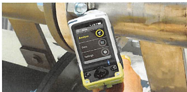
The Niton XL5 Plus analyzer in use, analyzing a tight weld in an oil refinery.
