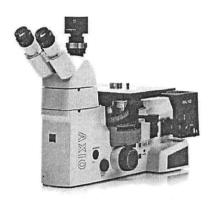
Zeiss Axiovert A1 MAT with Bright Field , Dark Field, and Polarized Light
